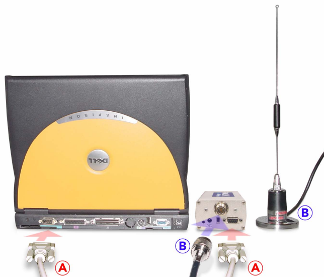
Figure 1. Serial port connection of ProRAE Remote Host Controller to modem (A) and modem to antenna (B).
